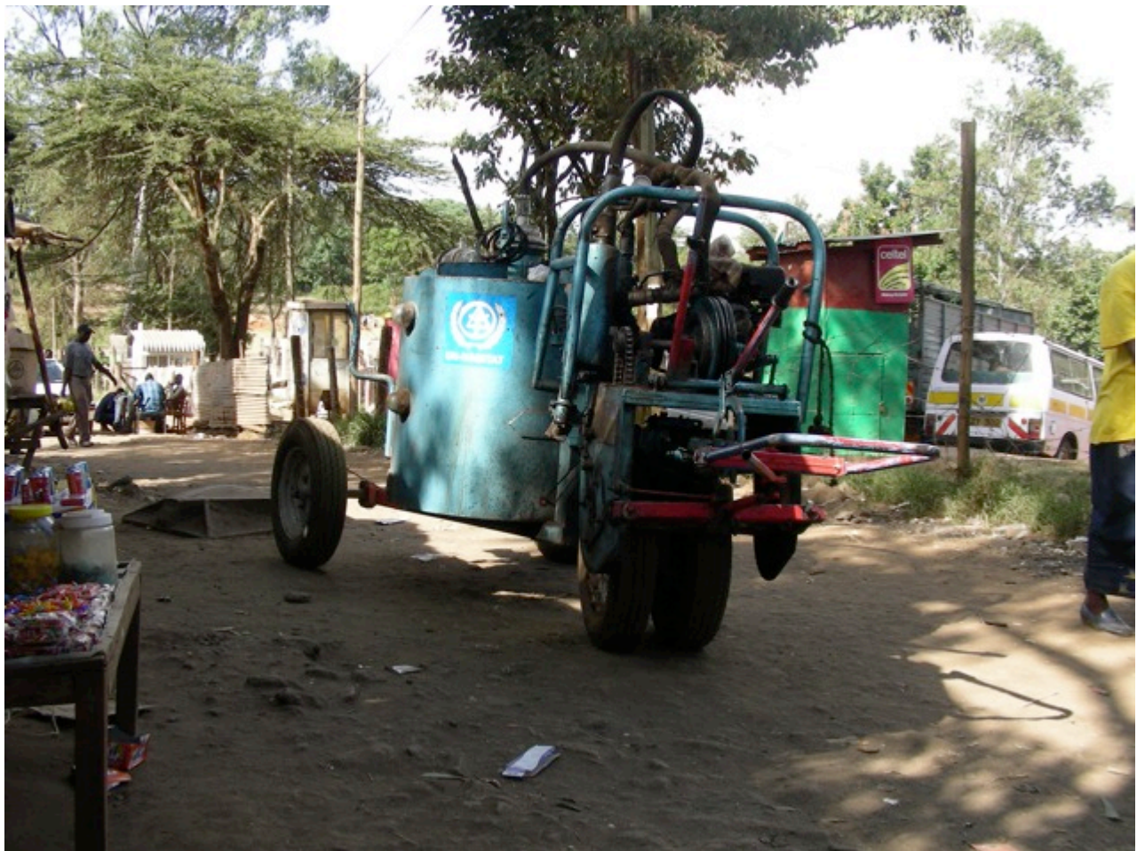
Photo 3 The UN HABITAT suction device is used for evacuating pit latrines, but it cannot work where access is limited.
